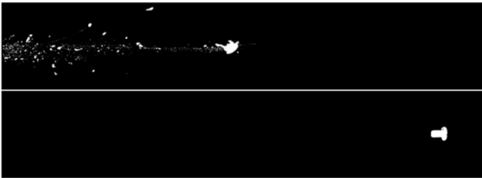
Courtesy Jeremy Roberts/Conservation Media X-ray images of lead (top) and non-lead (bottom) ammunition shot into a ballistics gel.
